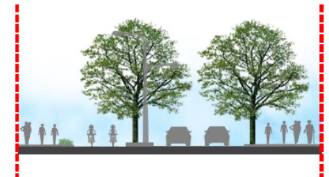
Typical Local Road Section: 17.9m ROW
